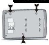
**Fig. 7:** Hook the front panel back on to the base of the box by re-inserting the hinges into their slots and making them bend.
