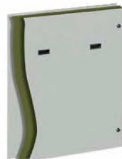
Sandwich soundproofing galvanized sheet panels, painted outside and isolated with high-density rock wool (100 Kg/m 3 )
